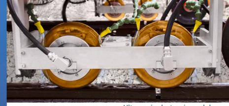
Ultrasonic electronic modules: OKOSCAN 73HS System employs ultrasonic single-channel modules OKO-24 with a frequency range of 1 to 7 MHz and PRF of up to 5 kHz.
