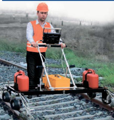
The flaw detector performs non-destructive testing of rails by pulse-echo, echo-mirror and mirror-shadow methods, using contact ultrasonic techniques. The ultrasonic testing provided by UDS2-73 is compliant with EN 16729-1 "Railway applications - Infrastructure - NDT on rails in track - Part 1: Requirements for ultrasonic inspection and evaluation principles", ETN-01-04 "Manual for Non-destructive Testing of rails" and other regulations.
