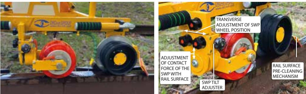
The positioning of each search wheel is accomplished through mechanical adjustments.
