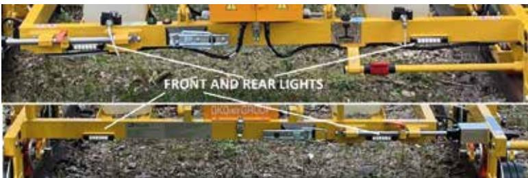
Illuminating the SWP wheel area simplifies the ultrasonic inspection process. The main directional lighting, which is placed on the retractable bar, significantly increases safety for personnel during ultrasonic inspections and provides long-range illumination of the direction of movement.
