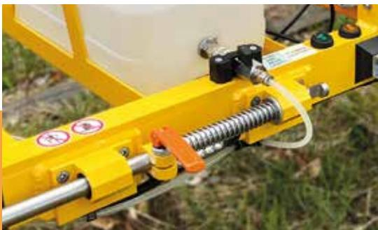
The design incorporates a system that constantly repeats the dynamic track gauge, ensuring that the search wheel (SWP) is always in the optimal position relative to the rail head during inspection.
